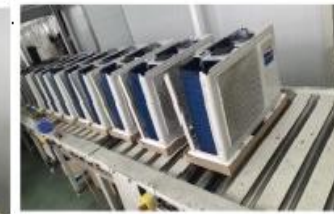
Heat pump production line
